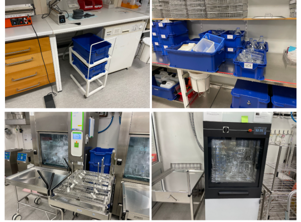
Fig. 1: Lab Automation use-case in the AstraZeneca chemical laboratories: a human operator drives a cart around the lab to collect dirty glassware, organizes it in a dishwasher tray, and finally inserts the tray in the dishwasher.
